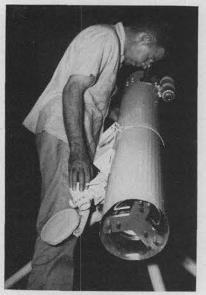
A FLASH SHOT catches Kenneth Kemp using his telescope in an evening observation of the Orion Nebula. Scope pictured here has a 6-inch mirror and is of a Newtonian type. Kemp is in 5214 and located at Salton Sea Base.
